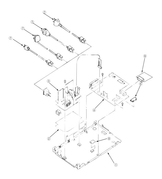
Figure 8-4 Base Plate Unit
